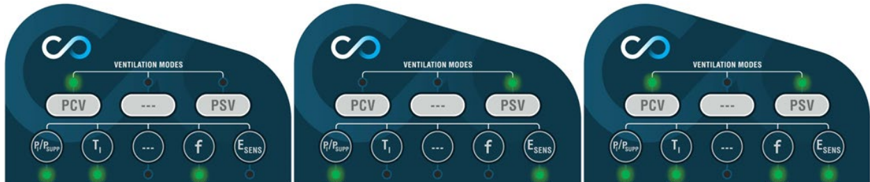
Backlit LED keys are used to elucidate relevant settings for user. A: PCV, B: PSV, C: SIMV (PCV+PSV)
